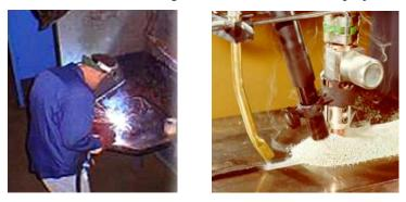
The Northrop Grumman Newport News-led team will investigate welding thick section HSLA-100 steel with Gas Metal Arc and Submerged Arc welding techniques using little or no preheat.
