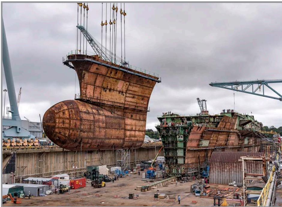
CVN 79 Lower Bow Positioned in Dry Dock. Courtesy of Huntington Ingalls Industries - Newport News Shipbuilding.
