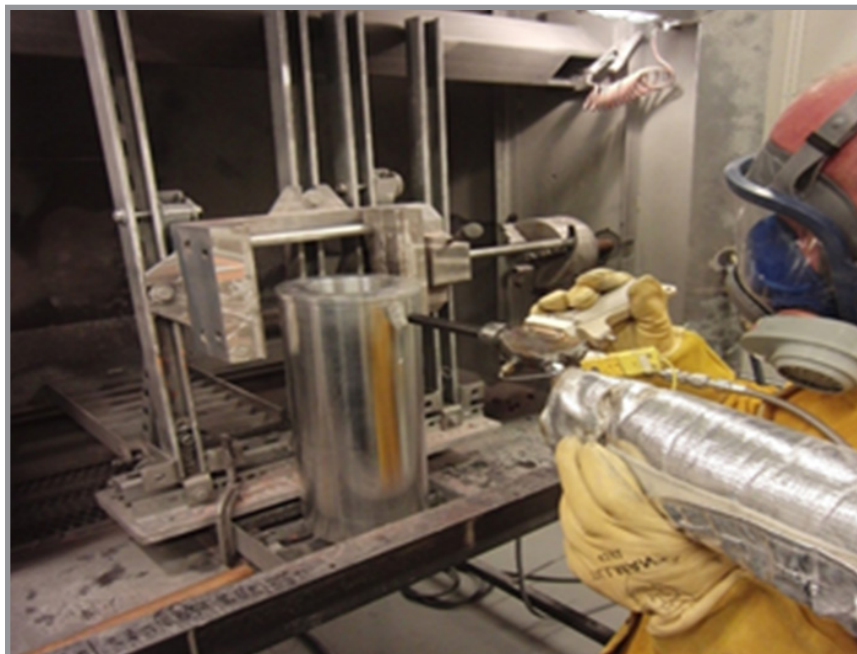
Innovative Cold Spray Repair Technology for Ships. Courtesy of iMAST.
